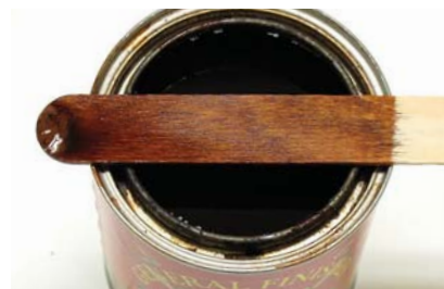
Pigment. General Finishes dye appears to contain pigment, which settles to the bottom of the can. Pigment requires a binder to glue it to the wood and, indeed, General Finishes contains an acrylic binder.
