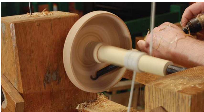
A hook. Here, I’m using one of the “dishturners’ tools,” specifically a hook, to hollow the inside of this bowl. The lathe’s power cord is wrapped around a mandrel fitted into the bowl.
