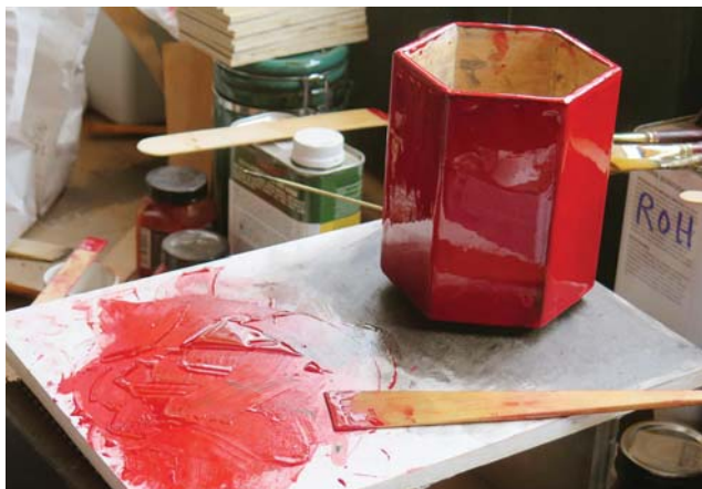
Red epoxy. This epoxy batch is mixed with red pigment powder and will be applied over the black base and the first red coating.
