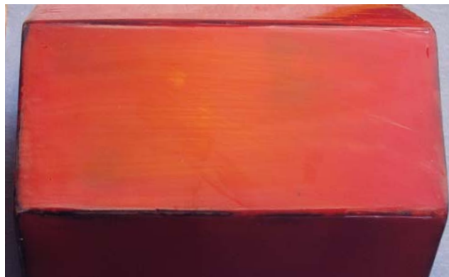
Scrape & sand. Here's how it looks scraped with a razor blade and sanded with #1,500-grit wet/dry paper and a sanding block.
