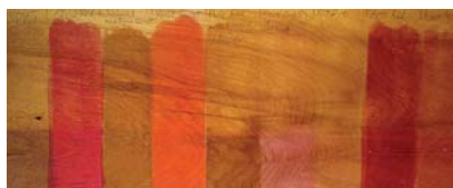
All dyes fade. I covered the bottom half of this panel and placed it in a west-facing window for six months. All the dyes faded (top half), some less than others, but they all faded. Use pigment to avoid fading in sunlight.
