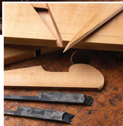
No. 6 pair. The details on J. Wilding's hollows and rounds are rooted in 19th-century British planes – simple and functional.
