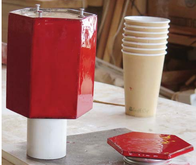
Freshly done. Here's the final pigmented faux urushi all freshly done. It will flow out a little in a half-hour or so.
