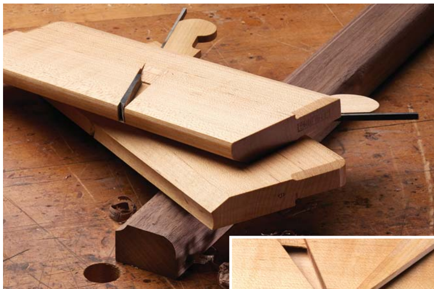
No. 6 pair. The details on J. Wilding's hollows and rounds are rooted in 19th-century British planes – simple and functional.
